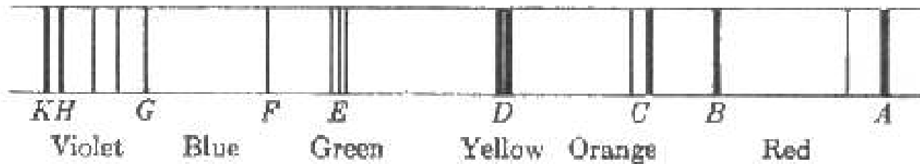
Figure 30.5 The Fraunhofer dark lines in the visible part of the solar spectrum. Only a few of the most prominent lines are represented here.
